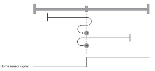
Figure 4-26 Homing mode 20 trajectory and signal status
