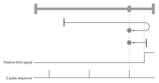
Figure 4-10 Homing mode 2 trajectory and signal status
