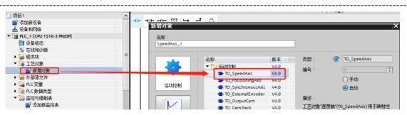
(2) In the "Hardware Interface" of the TO axis configuration, select "PROFIdrive" as the "Drive Type" input. Select the desired X5E(F)R as the "Drive".
