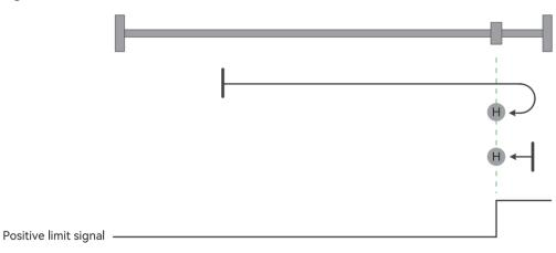
Figure 4-24 Homing mode 18 trajectory and signal status
