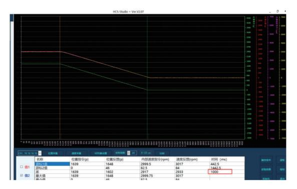
Similarly, the time taken to trigger the disable and interrupt IntermediateStop pins is 1s.
