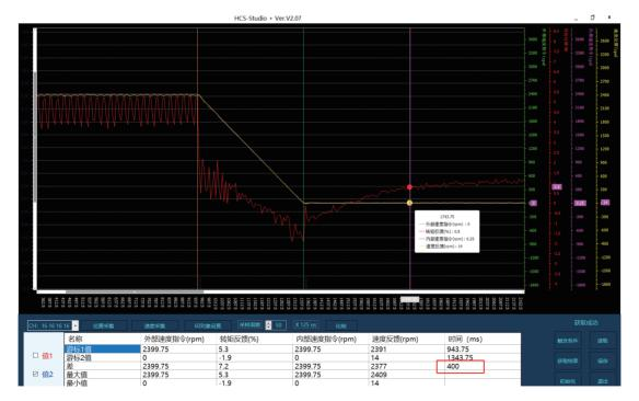
Based on the above, change OverAcc and OverDec to 80 and 50 respectively, Jog acceleration time (s) =  $(3000000^*80\%) / (50000^*60^*80\%) = 1$  (s), jerk deceleration time (s) =  $(3000000^*80\%) / (100000^*60^*50\%) = 0.8$  (s).
