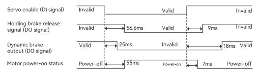
The timing of "Holding brake release signal" during the servo OFF is related to the motor running speed, see the parameter description for details, and the minimum value is 9ms.
