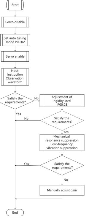
Fig. 3.3 Automatic gain adjustment flow
