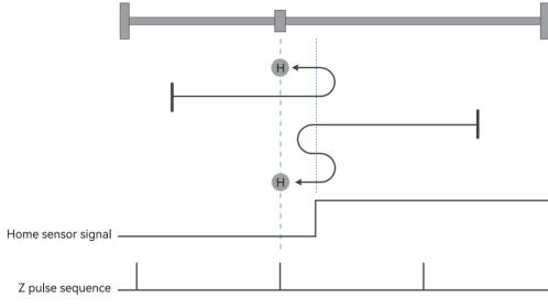
Figure 4-11 Homing mode 3 trajectory and signal status
