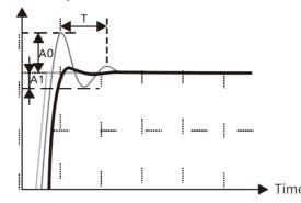
Fig. 3.10 Low frequency vibration waveform during positioning control
