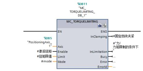
Description: The motion control instruction "MC\_TorqueLimiting" activates and specifies the parameters for torque/ torque limiting and fixed block detection. Fixed block detection enables motion operations such as "motion to fixed block" and position control. In the axis configuration, it is possible to configure whether the force/torque limit is related to the drive side or the load side (step 3). The "MC\_TorqueLimiting" block is only supported with messages 102 and 105. Parameter:
