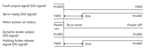
The timing of the "Holding brake release signal" during the faulty stop is related to the servo parameters P04.52 and P04.53 and the motor running speed, see the parameter description for details, and the minimum value is 2ms.
