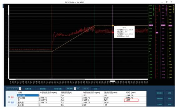
The waveform of the jog deceleration time is shown as:
