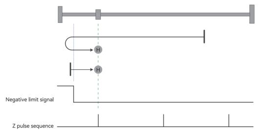
Figure 4-9 Homing mode 1 trajectory and signal status
