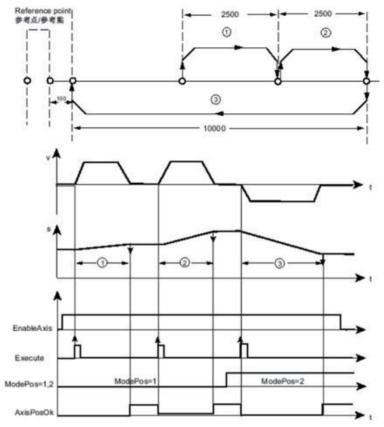
Absolute positioning mode control timing
