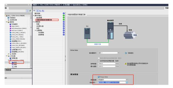
(3) Drag out the torque limit FB ino the program area (MC\_TORQUERANGE).
