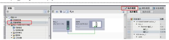
(2) Open the device properties by double-clicking on the X5FR image. Select the Isochronous Mode checkbox in the Isochronous Mode option to activate IRT mode:
