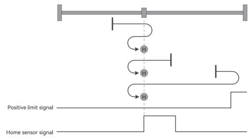
Figure 4-30 Homing mode 24 trajectory and signal status
