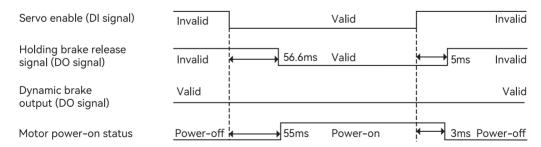
The timing of "Holding brake release signal" during the servo OFF is related to the setting of servo parameter P04.52 and P04.53 and the running speed of the motor, see the parameter description for details, and the minimum value is 5ms.
