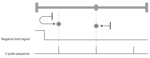
Figure 4-37 Homing mode 33 trajectory and signal status
