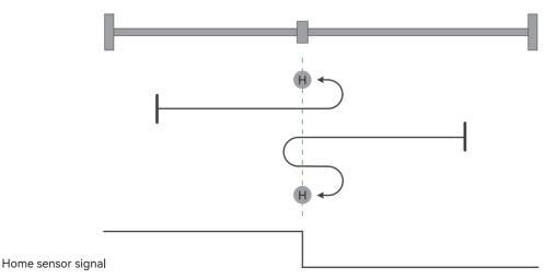
Figure 4-28 Homing mode 22 trajectory and signal status
