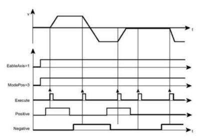
Continuous operation mode control timing
