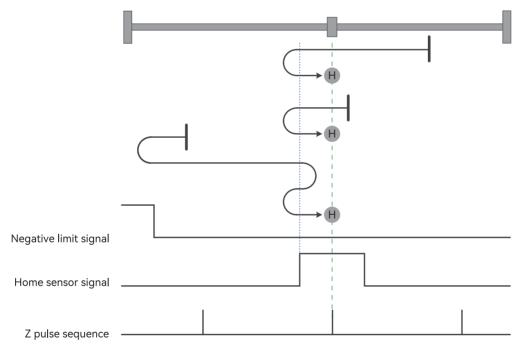
Figure 4-21 Homing mode 13 trajectory and signal status
