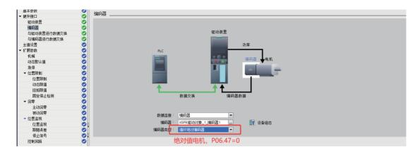
(5) Set "Data exchange with inverter" to exchange data with the drive: Users can check the box to automatically apply the drive value during operation.
