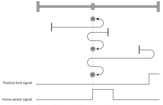
Figure 4-29 Homing mode 23 trajectory and signal status
