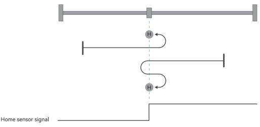
Figure 4-25 Homing mode 19 trajectory and signal status
