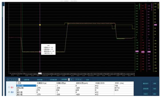
High-speed homing speed is 500RPM homing low speed is 30RPM and homing acceleration time = 5000000/ (60\*1000000)=0.0833s,
