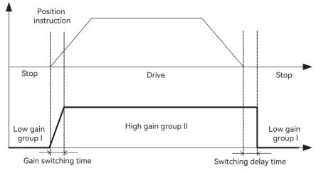
Fig.3.4 Example of gain switching
