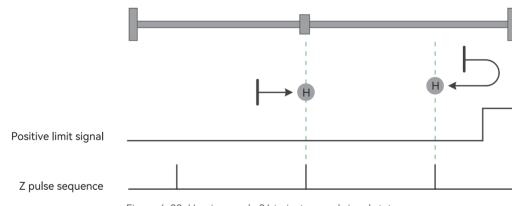
Figure 4-38 Homing mode 34 trajectory and signal status
