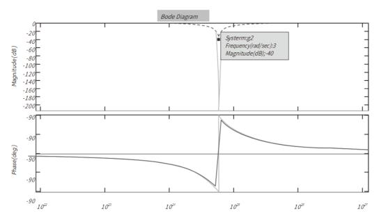
Figure 3.7 Frequency domain response curves when the depth of the notch filter is set to 1 and 0, respectively
