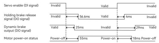
The timing of "Holding brake release signal" during the servo OFF is related to the motor running speed, see the parameter description for details, and the minimum value is 4ms.
