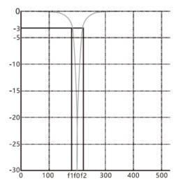
Fig.3.6 Notch filter amplitude-frequency characteristics
