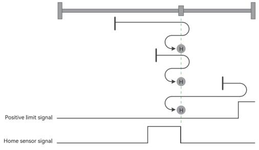
Figure 4-32 Homing mode 26 trajectory and signal status
