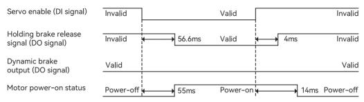
The timing of "Holding brake release signal" during the servo OFF is related to the motor running speed, see the parameter description for details, and the minimum value is 4ms.
