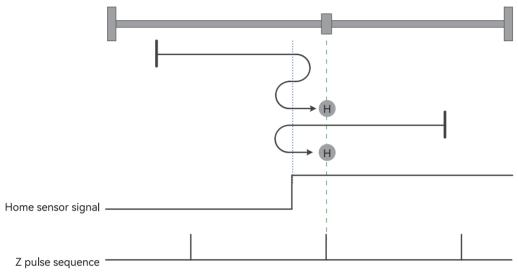
Figure 4-12 Homing mode 4 trajectory and signal status
