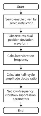
Fig. 3.11 Operation flow of low-frequency suppression function
