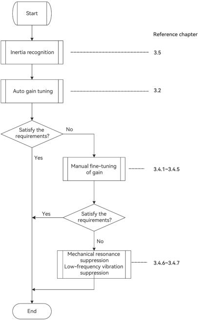
Fig. 3.2 Gain tuning process
