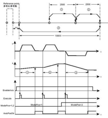
Relative positioning mode control timing
