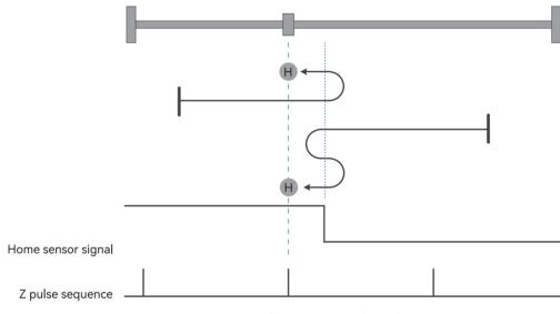
Figure 4-14 Homing mode 6 trajectory and signal status
