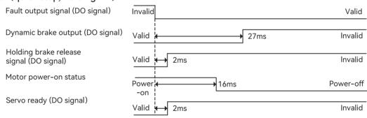
The timing of the "Holding brake release signal" during the faulty stop is related to the motor running speed, see the parameter description for details, and the minimum value is 2ms.
