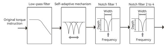
Fig. 3.8 The role of the notch filter in servo control
