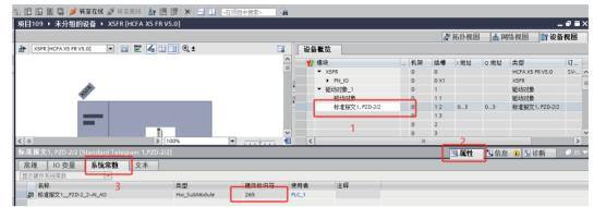
3. Drag SINA\_Speed (FB285) function block into the programming network in OB1 and populate the HWIDSTW and HWID-ZSW pins with the hardware identifiers.
