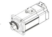
When viewed from the front of the flange, the shaft turns back in the counterclockwise direction, i.e., CCW.
