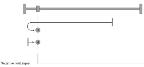
Figure 4-23 Homing mode 17 trajectory and signal status
