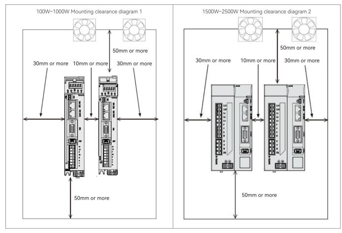
• The drive can be installed only in the vertical direction. During installation, use two M4 screws to fix the drive with an output power of 750W or less. Use three M5 screws each to secure the drive with an output power of 1kW or more and the main drive when installing them.
