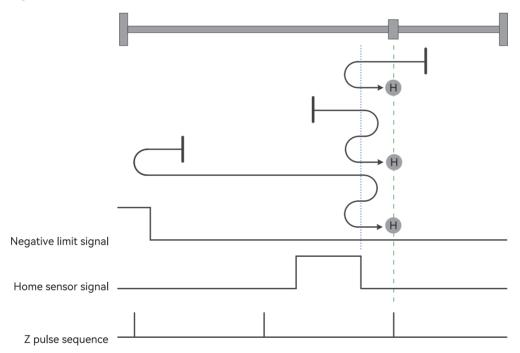
Figure 4-19 Homing mode 11 trajectory and signal status
