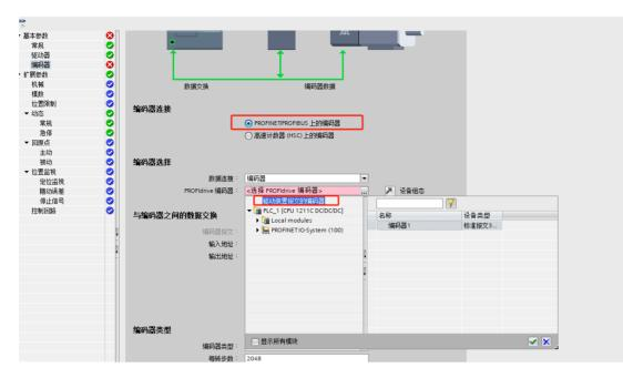
(2) After selecting the encoder connection method, it needs to configure the encoder type (rotary incremental or rotary absolute), as well as the encoding parameter settings, users can check the automatic uploading, the following figure shows the automatic uploading of incremental motor.
