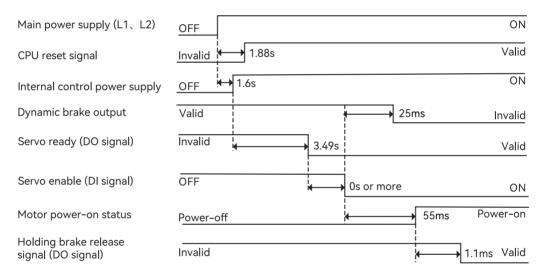
Servo enable on and off action during motor rotation
