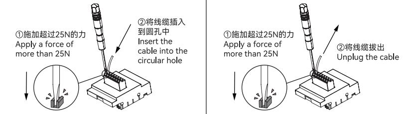
EN During connecting, insert the flat-blade screwdriver into the unlocking tab of the terminal with a force of more than 25 N. Then insert a cable into the circular hole. Gently tug the cable after pulling out the screwdriver. If the cable is secured firmly, then the connection is finished. The reverse is the procedure for unplugging the cable. The terminal specifications and wiring diagram are shown in the right figure.
