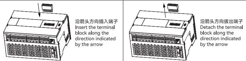
EN The mounting and dismounting of the removable terminal block are shown in the figures on the right side.
