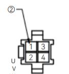
**X2M Power brake cable(for 400~750W models)**
