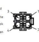
**X2M Power brake cable(for 100~200W models)**
